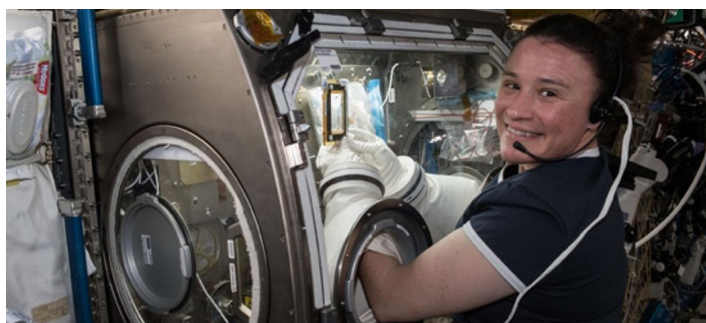
Figure 4: NASA astronaut Serena Auñón-Chancellor conducts research operations for the Angiex Cancer Therapy Study inside the Microgravity Science Glovebox (Left) and demonstrates the hardware (Right), Image Credit: NASA.
